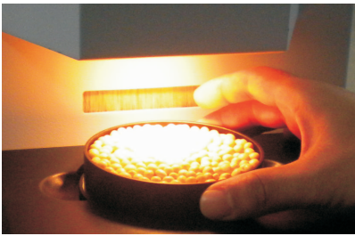
Rotary Sample plate leads to accurate analysis
